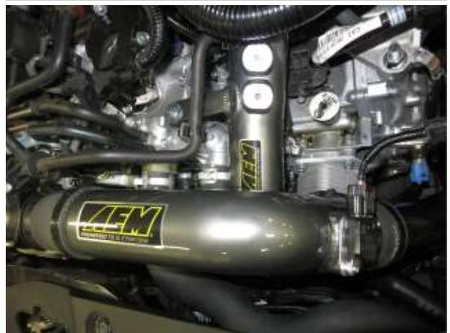
p. Reinstall the upper AEM intake tube. Make sure it does not contact the charge pipe. Finally, reconnect the MAF sensor harness.
