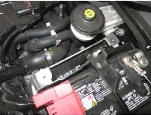
g. Use a 10mm socket to remove the (2) M6 bolts fastening the battery heat shield. Remove the heat shield. Do not discard these components.
