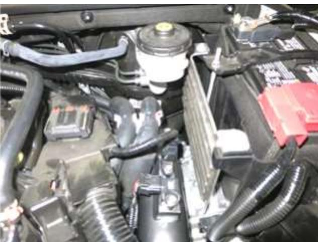
o. Reinstall the battery heatshield.
