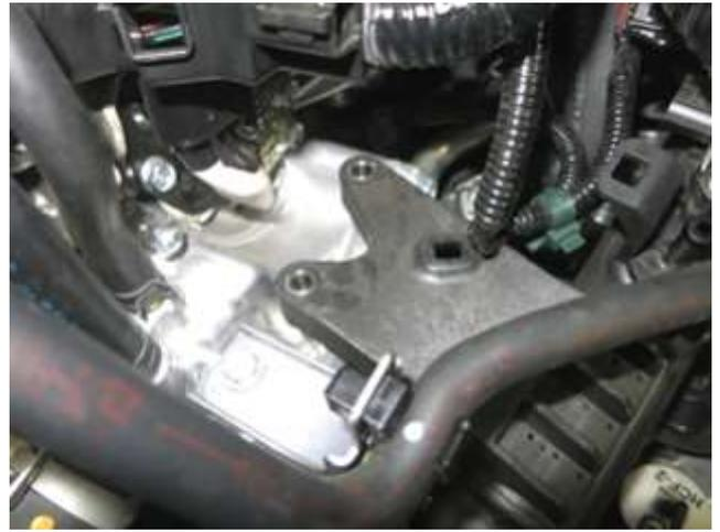
f. Use a 10mm socket to remove the (2) M6 bolts fastening the stock charge pipe to the engine block. Do not discard this hardware.
