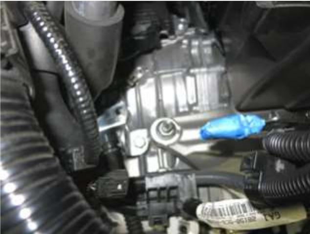
a. Before commencing the install of your AEM charge pipe, wrap the end of the bracket, shown above, in tape. This will protect the pipe from scratches as you maneuver it into place.
