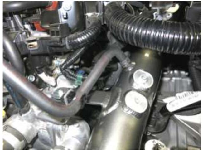
l. Install the vacuum hose to the nipple and secure with the factory spring clamp. Then, reattach the plastic clip to the mounting bracket.
