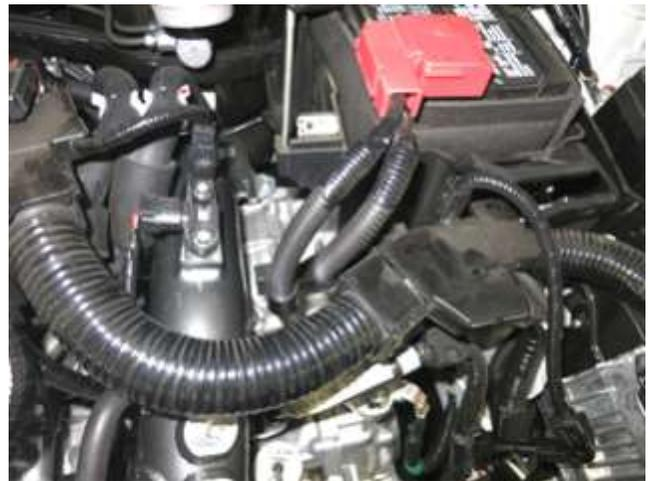
n. Reattach the (2) harnesses to the mounting bracket.
