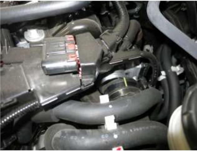
k. Loosen the hose clamp securing the charge pipe to the throttle body. Then, pull the hose end off of the throttle body.
